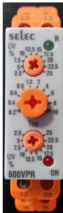
1 - Device front face showing Overvoltage, Time Delay and undervoltage Settings
